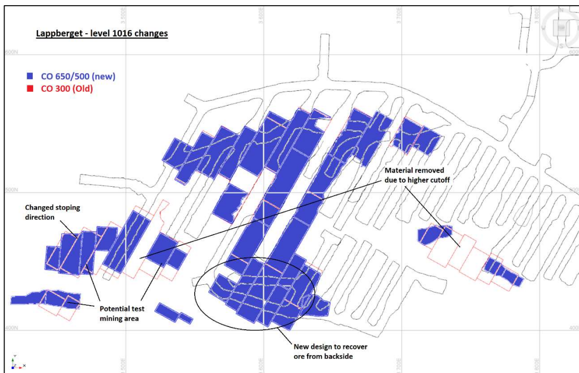
Figure 3-15. Illustration of differences caused by the cutoff change and new backside design on level 1016. The old design (red stopes) was completed using NSR cut-off of 300 SEK/t (20LTP22), which is equivalent to 410 SEK/t with 24LTP26 NSR values. The new design (blue stopes) was completed NSR using NSR 2023 cut-off of 650 SEK/t (24LTP26) allowing for pillars as low as 500 SEK/t.
