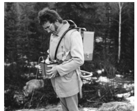
▲ Svante Holmqvist with an electrical prospecting instrument with a VLF receiver, 1973.
