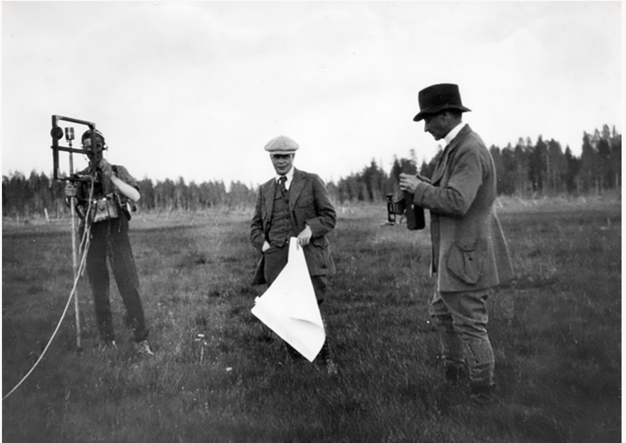
Twin frame Electromagnetic measurement in Mensträsk. Director Oscar Falkman on the right and engineer Karl Sundberg, center.
